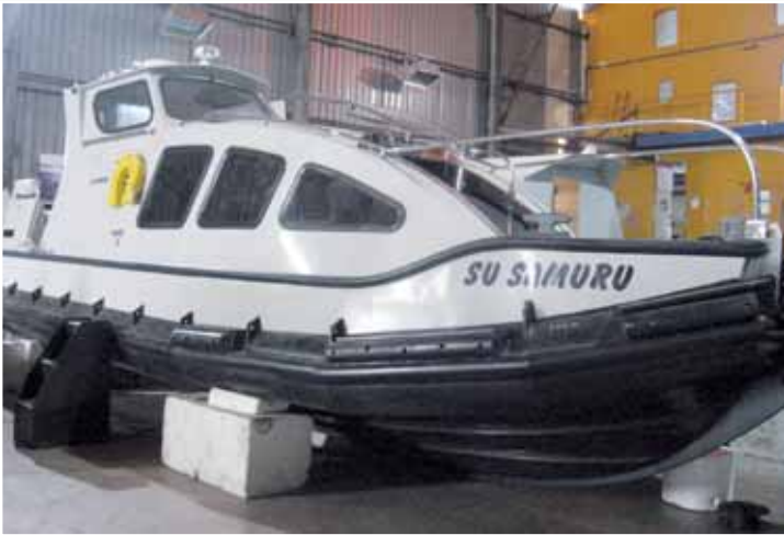
Ship constructed completely of HD-PE, Turkey
