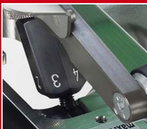
Adjustment of welding force for different materials
